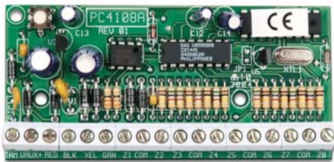
KT-PC4108 - 8-Zone Input Expansion Module
